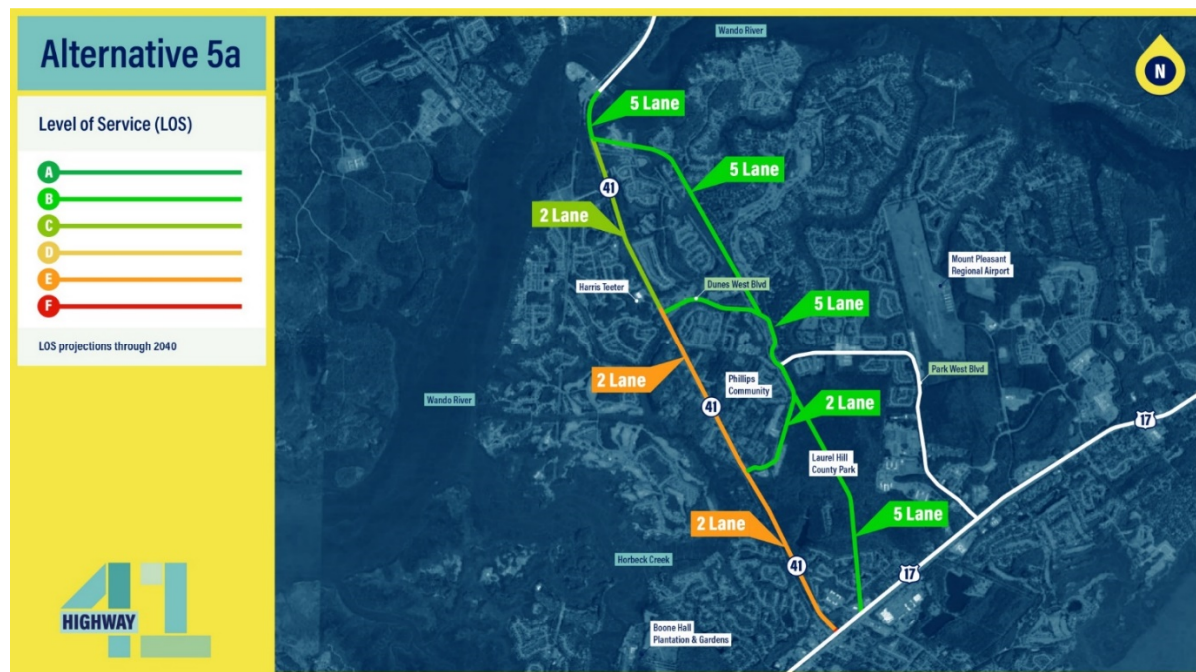
Figure 2. Level of Service for Alternative 5a
