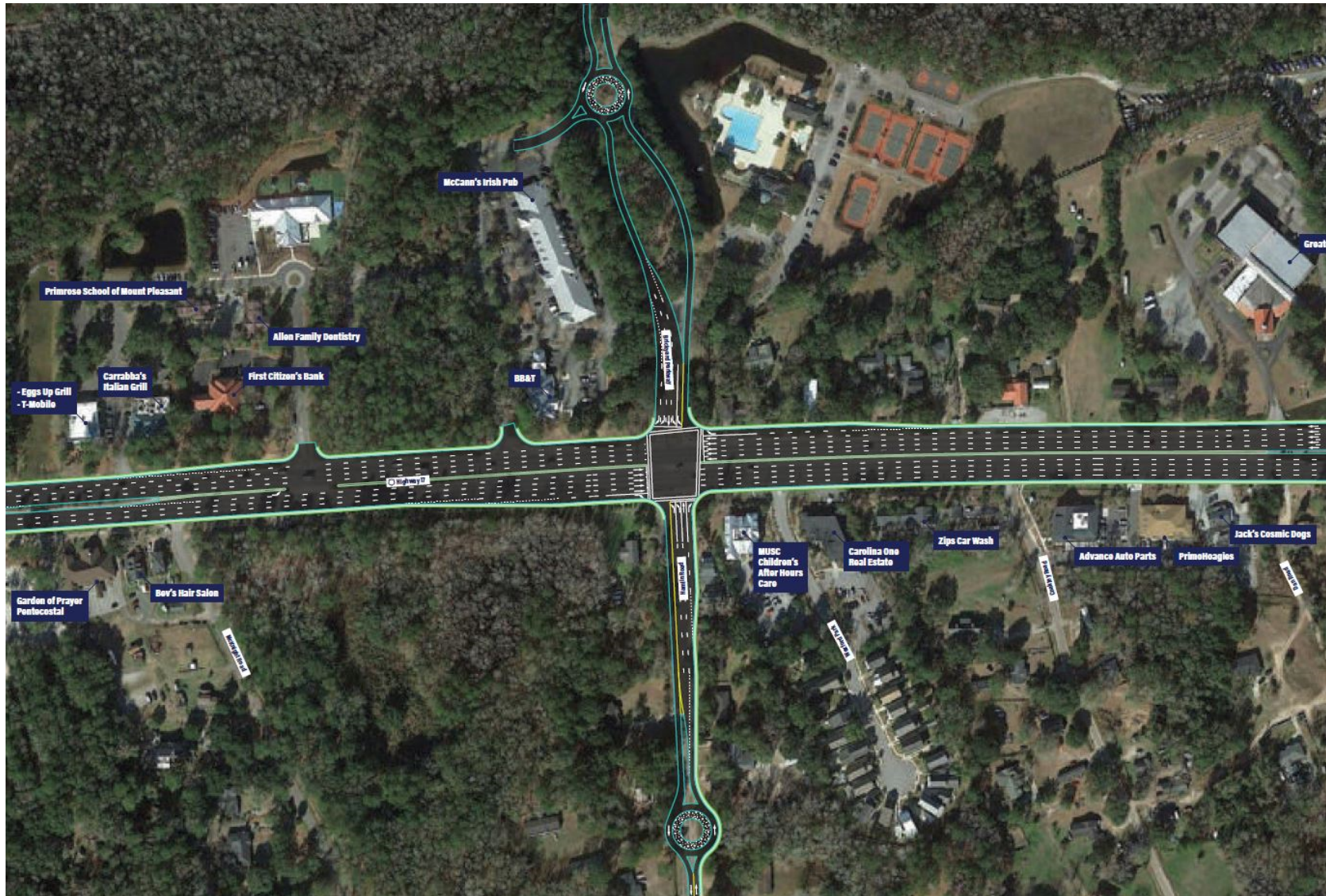
Figure 3-5. Design Concept – Brickyard Parkway/Hamlin Road and US 17 Intersection
