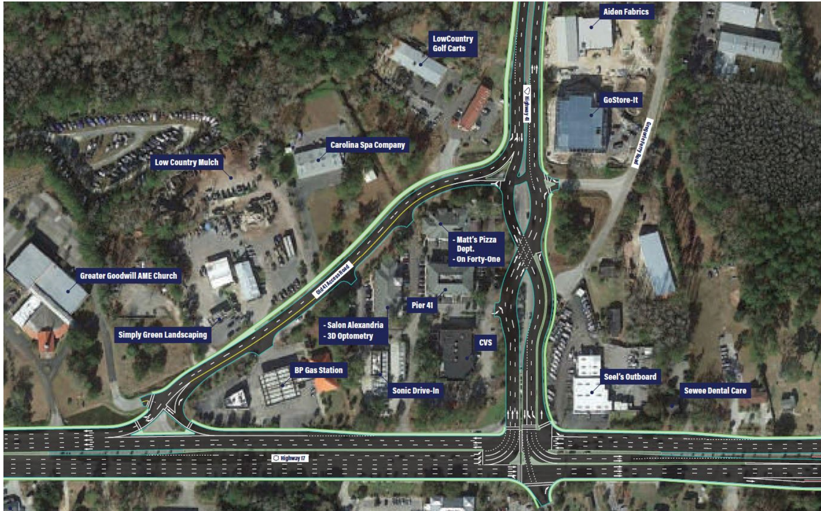
Figure 3-2. Design Concept – SC 41 and US 17 Intersection
